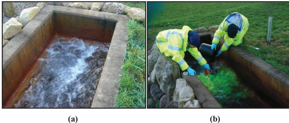
Figure 3.4 Example of (a) tracer injection point at the inlet of a treatment system (b) injection of Na-fluorescein dye and sodium bromide tracers
